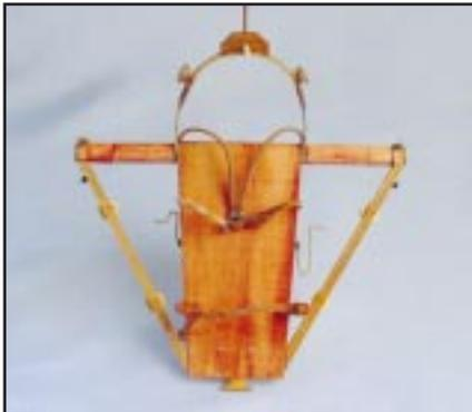
*Construction incorporates numerous individual elements, including a wing attachment harness that the modeler laminates on a male form.*
